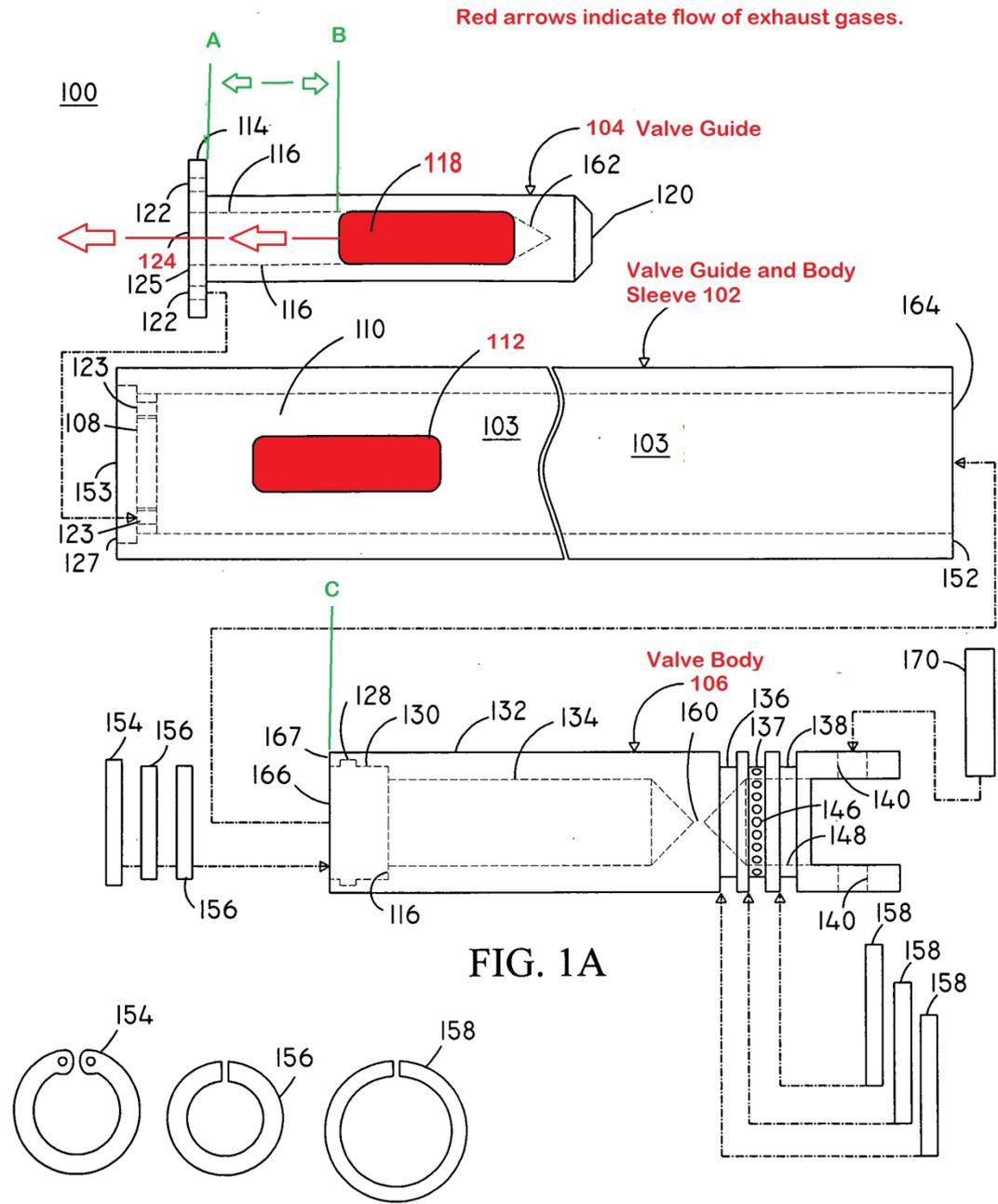
154 is a retaining ring that holds compression seal rings 156 in place. 158 are compression seal rings that also provide lubrication.
